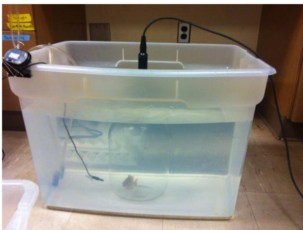
Figure 1: Experimental apparatus for measuring oxygen consumption in fish using a closed respirometer chamber (jar where fish is) fitted with an optical oxygen probe (horizontal object in front of the fish).
